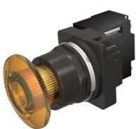
30mm BlackMax, Epoxy Coated Corrosion Resistant Metal Operator, Round Illuminated Twist-to-Release Full Voltage, 6V AC/DC Incandescent Lamp Mushroom Head Cap Small 1.79" (45 mm) Plastic Cap, Amber 2 Position Maintained, Twist-to-Release UL Listed, CSA Certified NEMA 1,3,3R,4,4X,12,13 & Automotive Standards
