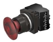
30mm BlackMax, Epoxy Coated Corrosion Resistant Complete Metal Unit Illuminated Twist-to-Release Full Voltage, 6V AC LED Lamp Mushroom Head Cap Small 1.79" (45 mm) Plastic Cap, Red 2 Position Maintained, Twist-to-Release with 1 N.O. - 1 N.C. Heavy Duty Contacts, A600/P600 UL Listed, CSA Certified NEMA 1,3,3R,4,4X,12,13 & Automotive Standards
