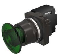
30mm BlackMax, Epoxy Coated Corrosion Resistant Metal Operator, Round Illuminated Twist-to-Release Full Voltage, 6V AC/DC Incandescent Lamp Mushroom Head Cap Small 1.79" (45 mm) Plastic Cap, Green 2 Position Maintained, Twist-to-Release UL Listed, CSA Certified NEMA 1,3,3R,4,4X,12,13 & Automotive Standards
