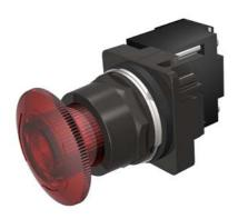
30mm BlackMax, Epoxy Coated Corrosion Resistant Metal Operator, Round Illuminated Twist-to-Release Full Voltage, 6V AC/DC Incandescent Lamp Mushroom Head Cap Small 1.79" (45 mm) Plastic Cap, Red 2 Position Maintained, Twist-to-Release UL Listed, CSA Certified NEMA 1,3,3R,4,4X,12,13 & Automotive Standards
