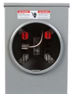
Siemens Low Voltage Talon Meter Sockets Residential - Talon Meter Sockets UAT1 Steel are Residential Enclosures Single-Family Metering. Type: UAT1 Special Features: NO BYPASS Application: RESIDENTIAL Standard: UL Voltage Rating: 300V Amperage Rating: 135A Phase: 1 OR 3 PHASE Size: 4.800X8.600X13.200 Cable Entry: UG Terminal: 5 TERMINALS Mounting: SURFACE MOUNTING Operating Temperature: AVERAGE AMBIENT Enclosure: STEEL
