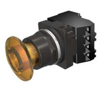
30mm BlackMax, Epoxy Coated Corrosion Resistant Complete Metal Unit Illuminated Twist-to-Release Full Voltage, 6V AC LED Lamp Mushroom Head Cap Small 1.79" (45 mm) Plastic Cap, Amber 2 Position Maintained, Twist-to-Release with 1 N.O. - 1 N.C. Heavy Duty Contacts, A600/P600 UL Listed, CSA Certified NEMA 1,3,3R,4,4X,12,13 & Automotive Standards
