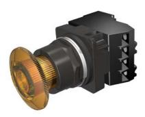
30mm BlackMax, Epoxy Coated Corrosion Resistant Complete Metal Unit Illuminated Twist-to-Release Full Voltage, 6V AC/DC Incandescent Lamp Mushroom Head Cap Small 1.79" (45 mm) Plastic Cap, Amber 2 Position Maintained, Twist-to-Release with 1 N.O. - 1 N.C. Heavy Duty Contacts, A600/P600 UL Listed, CSA Certified NEMA 1,3,3R,4,4X,12,13 & Automotive Standards
