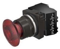
30mm BlackMax, Epoxy Coated Corrosion Resistant Complete Metal Unit Illuminated Twist-to-Release Full Voltage, 6V AC/DC Incandescent Lamp Mushroom Head Cap Small 1.79" (45 mm) Plastic Cap, Red 2 Position Maintained, Twist-to-Release with 1 N.O. - 1 N.C. Heavy Duty Contacts, A600/P600 UL Listed, CSA Certified NEMA 1,3,3R,4,4X,12,13 & Automotive Standards
