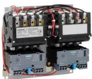
2-speed 3-phase motor starter Size 4 Two separate windings Constant or variable torque Solid-state overload relays Low SPD OLR range 50-200A High SPD OLR range 50-200A 110V 50HZ / 120V 60HZ coil Enclosure NEMA type (open) No enclosure
