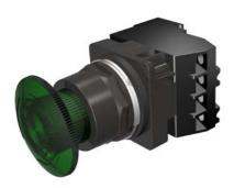
30mm BlackMax, Epoxy Coated Corrosion Resistant Complete Metal Unit Illuminated Twist-to-Release Full Voltage, 6V AC/DC Incandescent Lamp Mushroom Head Cap Small 1.79" (45 mm) Plastic Cap, Green 2 Position Maintained, Twist-to-Release with 1 N.O. - 1 N.C. Heavy Duty Contacts, A600/P600 UL Listed, CSA Certified NEMA 1,3,3R,4,4X,12,13 & Automotive Standards
