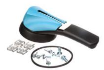
Siemens Low Voltage Circuit Protection OEM Disconnect & Accessories. Type 1, 3R, 12, 4/4X rotary operating handle (door mounted) blue and black. Compatibility: (CFSS5200HN, CFSS5400HN, CFSS10200HN, CFSS10400HN shafts), (30 - 400A switches). Special features: heavy duty pistol grip 4.92 IN long, defeatable cover interlock provided. Cover cannot be opened when handle is padlocked in the OFF position.
