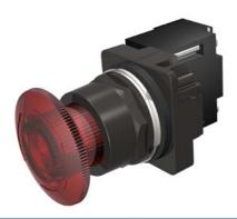
30mm BlackMax, Epoxy Coated Corrosion Resistant Metal Operator, Round Illuminated Twist-to-Release Full Voltage, 6V AC LED Lamp Mushroom Head Cap Small 1.79" (45 mm) Plastic Cap, Red 2 Position Maintained, Twist-to-Release UL Listed, CSA Certified NEMA 1,3,3R,4,4X,12,13 & Automotive Standards
