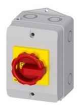
SENTRON, Switch disconnector 3LD, emergency switching-off switch, 3- pole, lu: 16 A, operating power / at AC-23 A 400 V: 7.5 kW, Molded plastic encapsulation for inch cable gland, rotary operating mechanism, red/yellow
