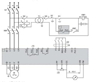
A1: ATV 212 drive KM1: Contactor Q1: Circuit breaker
