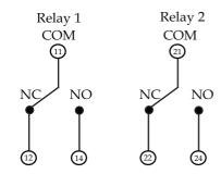
Note- Relay Contacts are shown in power off condition
