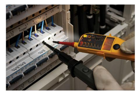
Fluke T90 Fluke T90 Voltage/Continuity Tester
