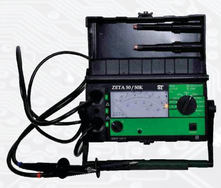
**Zeta** 50/50K Is used for the non-destructive measurement of insulation resistance in electrical systems, at machines, transformers and cables.
