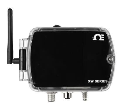
The XW Series Transmitters provide a wireless interface to a range of digital probes, digital I/O, and analog process signals. The radio is an IEEE 802.15.4 compliant transmitter operating at 2.4 GHz designed to transmit up to 1000 m\* (3280') and 100 m\* (328') to a ZW-REC coordinator.
