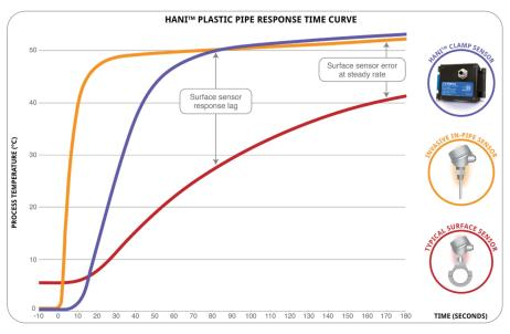
1. t63 is the time constant or response time required to reach 63.2 % of the final value after an instantaneous temperature change. t90 is the response time required to reach 90 % of the final value after an instantaneous temperature change.
