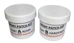
Applications include sealing rivets, bolts, metal joints, seams and welds, cement cracks, pipe couplings, joints and tees. Each kit has two containers of material and application instructions. When the resin and hardener are mixed, a gray epoxy is formed which cures at room temperature, has high adhesion and will not sag. It is resistant to oils, acids and chemicals.
