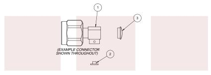
1. STRIP CABLE AS SHOWN, CHAMFER CENTER CONDUCTOR AND DEBURR CABLE.
