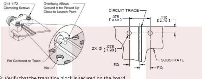
Step 3: Verify that the transition block is secured on the board.
