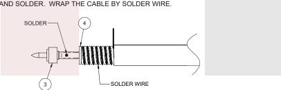
3. PUSH THE CONNECTOR BODY INTO THE CABLE, UNTIL IT STOPS. SOLDER THE CONNECTOR BODY WITH CABLE AND COVER HEATSHRINK SLEEVE.
