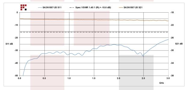
20 dB Fixed Attenuator N Male To N Female Up To 3 GHz Rated To 100 Watts With Black Aluminum Heatsink Body from Fairview Microwave is in-stock and available to ship same-day. All of our RF/microwave products are available off-the-shelf from our ISO 9001:2008 certified facilities in Lewisville, Texas. Fairview Microwave is RF on-demand.
