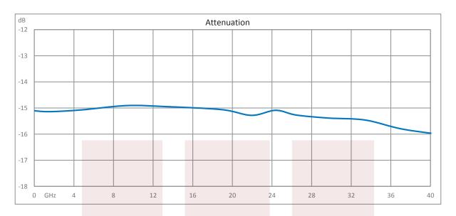
15 dB Fixed Attenuator 2.92mm Male To 2.92mm Female Up To 40 GHz Rated To 0.5 Watts With Passivated Stainless Steel Body from Fairview Microwave is in-stock and available to ship same-day. All of our RF/microwave products are available off-the-shelf from our ISO 9001:2008 certified facilities in Allen, Texas. Fairview Microwave is RF on-demand.
