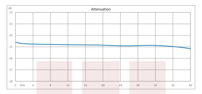
15 dB Fixed Attenuator 2.92mm Male to 2.92mm Female Up to 40 GHz Rated to 1 Watt with Passivated Stainless Steel Body from Fairview Microwave is in-stock and available to ship same-day. All of our RF/microwave products are available off-the-shelf from our ISO 9001:2008 certified facilities in Allen, Texas. Fairview Microwave is RF on-demand.
