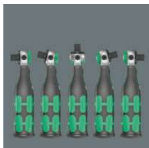
The ratchet head pivots freely and can be locked into any defined position by using the slide switch that is positioned on either side. It is even possible to work in very confined and difficult-to-access areas with enhanced hand clearance. The predefined locking at 0°, 15° and 90°, both to the right and left, ensure safe working without any slipping of the ratchet head.
