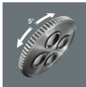
The fine tooting with 72 teeth allows for a low return angle of only 5° for working in constricted screwdriving situations.
