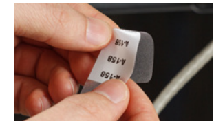
Fold flap behind printed area at perforated line, then apply to wire.
