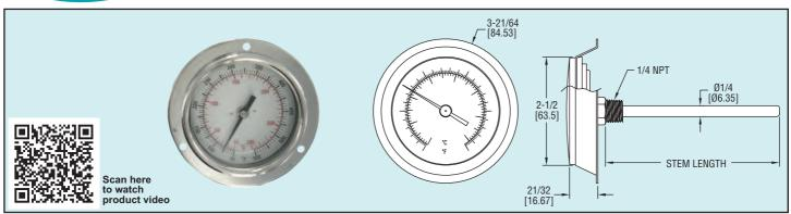
Series BTPM Panel Mount Bimetal Thermometers are designed to easily mount in most instrument panels. The front flange has three 5/32" diameter holes to quickly attach the thermometer to the panel. The Series BTPM thermometer has a 3" dial with a scratch resistant glass lens. The Series BTPM Panel Mount thermometers are ideal for HVAC, automotive, and food industry applications, chemical operations, and more.
