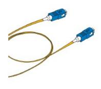
Single mode patch cords are used for telecom networks and also used for high speed metropolitan and access network. The single mode patch cords are manufactured using LSZH cables which conform to IEC, EIA TIA or Telcordia standards. The OS2 enhanced patch cords are terminated with optimized connectors which give optimum optical performance.
