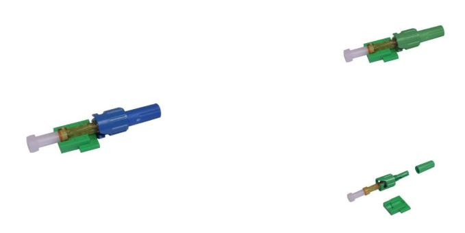
ST field installable connectors (FIC) are factory terminated and polished to make fiber terminations fast, easy and reliable. These fiber optic connectors offer terminations in less than 2 minutes without any difficulty and require no epoxy, polishing or crimping. The FIC greatly reduces the installation and set up time. It has a window feature to allow testing with a visual fault locator.
