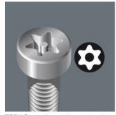
**TORX®** tools with a borehole unauthorised prevent the unfastening of safety screws. The screws contain a pin that protrudes into the drive profile so that "normal" TORX® tools cannot be used. This pin fits into the borehole of TORX® BO tools allowing safety screws to be unfastened.
