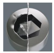
Hexagon screws can endure a problem because the contact surfaces delivering the power from conventional tool, transferred to the screw via very surface areas. consequence: the screw can become damaged (rounding out). Hex-Plus tools have a greater contact surface that prevents this from happening! At the same time, as much as 20 % more torque can be applied. Good to know: Hex-Plus tools fit into every standard hexagon socket screw!
