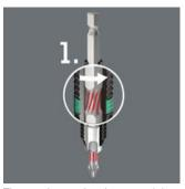
The torsion spring integrated into unique BiTorsion holder the absorbs lower levels of peak loads (Phase 1). Any overloading of this spring is effectively prevented by means of а supporting mechanism.
