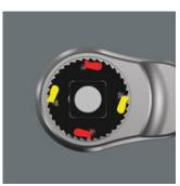
The dual-ratchet-teeth design means that a 76 fine-toothing division can be achieved from the 38 robust teeth with a return angle of only  $4.7^{\circ}$ .
