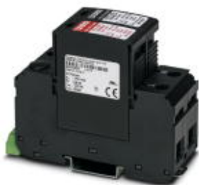
Surge protective device, two channel with remote indicator contact for 120 V AC, 2-wire plus ground.
