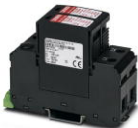
Surge protective device, two channel with remote indicator contact for 120/240 V split phase AC, 3-wire.
