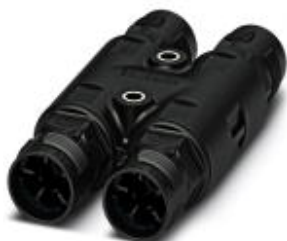
H distributor, QUICKON connection, number of positions: 4+PE, 0.5 mm 2 ... 1.5 mm 2 , 690 V, 17.5 A, black, Without QUICKON nut
