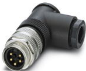
Connector, 4-position, Plug angled 7/8"-16UNF, Screw connection, knurl material: Zinc die-cast, nickel-plated, cable gland Pg13,5, external cable diameter 10 mm ... 12 mm, Contact 4 leading
