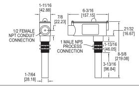
The **MODEL CLS1** Capacitance Level Switches provides reliable point level measurement of solids, liquids and slurries in metallic or non-metallic tanks and vessels. It detects the presence or absence of material in contact with the probe by sensing a change in the capacitance.
