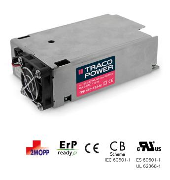
The TPP 450 Series of 450 Watt AC/DC power supplies feature a reinforced double I/O isolation system according to latest medical safety standards (60601-1 3rd edition, 2 × MOPP). The earth leakage current is below 100  $\mu$ A what makes the units suitable for BF (body floating) applications. The excellent efficiency of up to 94% allows a high power density for the standard 3" x 5" packaging format.
