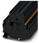
Fuse modular terminal block, fuse type: Glass / ceramics / ..., connection method: Push-in connection, cross section: 0.5 mm<sup>2</sup>- 10 mm<sup>2</sup>, AWG: 20 - 8, nominal current: 10 A, nom. voltage: 250 V, width: 8.2 mm, fuse type: G / 6,3 x 32, mounting type: NS 35/7,5, NS 35/15, color: black
