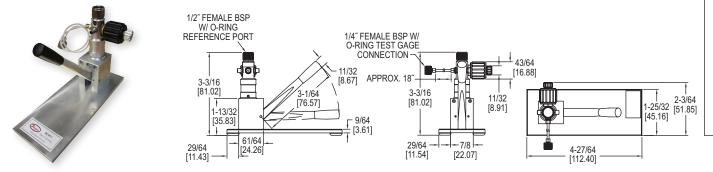
The **SERIES BCHP** Low Pressure Calibration Pump is able to generate pressure and vacuum for adjusting or calibrating pressure gauges, transmitters, or switches. The pump is hand operated and has a pneumatic pressure range of -28 to 870 psi (-0.95 to 60 bar).
