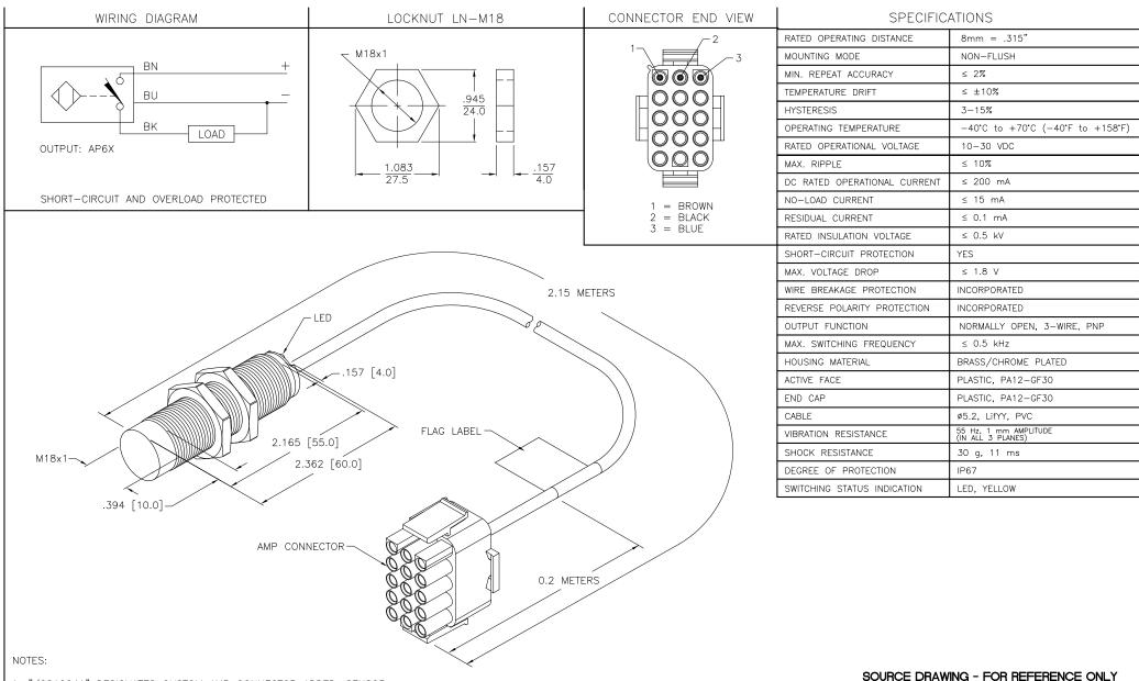
1. "/CS12241" DESIGNATES CUSTOM AMP CONNECTOR ADDED. SENSOR RATÉD TO -40°C. 2.15M TOTAL LENGTH FROM END TO END. FLAG LABEL 200MM FROM FRONT OF CONNECTOR.
