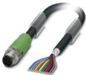
Sensor/actuator cable, 12-position, PUR/PVC, black RAL 9005, shielded, Plug straight M12 SPEEDCON, A-coded, on free cable end, cable length: 5 m
