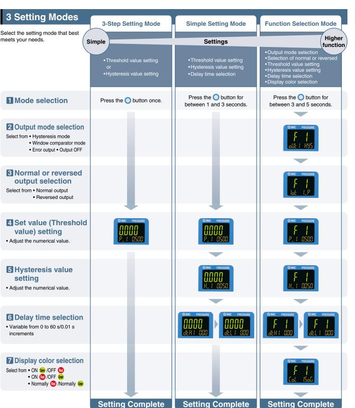
\* The chart above shows OUT1 operations. The Function Selection Mode for OUT2 is set using "F2." "2" will be displayed instead of "1" in the illustration above. (Example) P\_1 → P\_2
