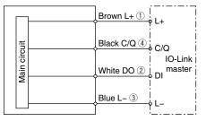
$\ast~$  The numbers in the circuit diagrams show the connector pin layout.
