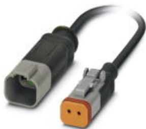
Sensor/actuator cable, 2-position, PUR halogen-free, black-gray RAL 7021, Plug straight DEUTSCH DT04-2P Clip locking, on Socket straight DEUTSCH DT06-2S Clip locking, cable length: 0.6 m
