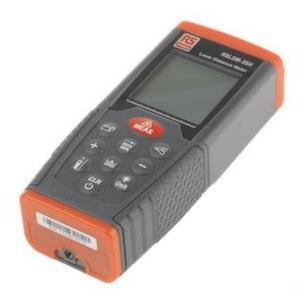
± 1.5 mm Accuracy Battery Life Up to 4000 Display Type LCD Imperial or Metric Both Laser Class Class 2 635 nm Laser Wavelength Measurement Range 0.05 to 35 m Model Number (p) RSLDM-35H Power Source Battery Weight 100 g
