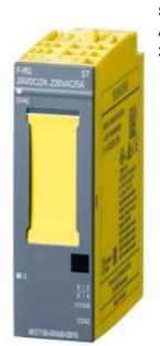
SIMATIC DP, Electronics module f. ET200SP, F-RQ 1x 24 V DC/24..230VAC/5A ST, 20 mm overall width, 1 relay output (2 NO) Summation output current 5 A, load voltage 24 V DC and 24.. 230 V AC, Can be used up to PL E (ISO 13849-1: 2008)/ SIL 3 (IEC 61508: 2010) if control takes place by (e.g. 6ES7136-6DB00-0CA0) F-DQ
