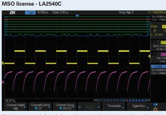
The I6 integrated digital channels are displayed along-side analog channels allowing users to view up to 18 time-correlated channels with shared triggering and acquisition on one screen. The LA2540C license enables the I6 digital channels of the 2540C Series and is included with MSO models.
