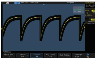
Perform up to 60,000 pass/fail decisions a second. Easy to generate masking templates help capture anomalies even with complicated waveforms.
