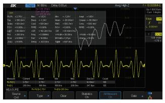
Display 36 automated measurements that include voltage, time, and statistics. Arithmetic and FFT functions can be performed on analog channels and two reference signals.
